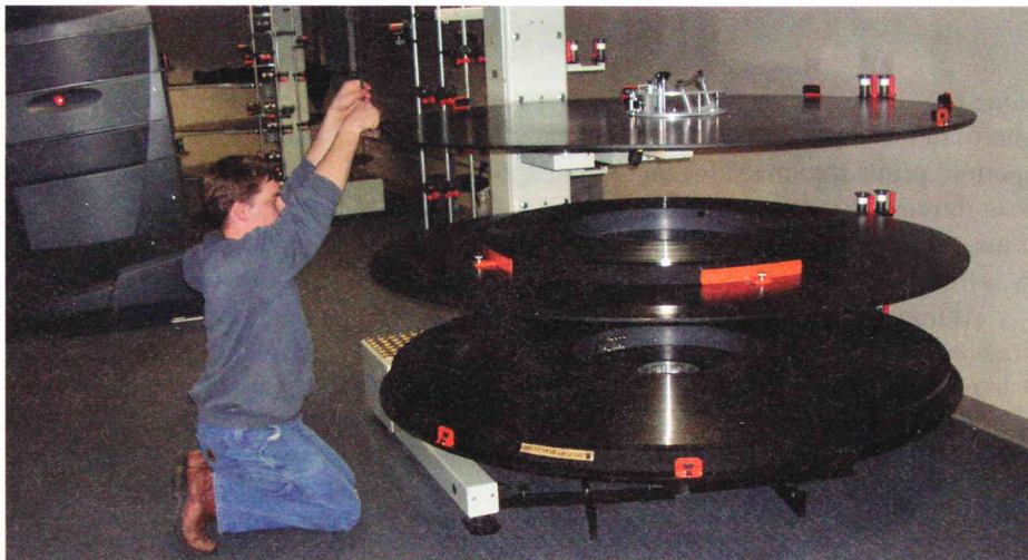
1.18 Most multiscreen theaters use platter projection, which winds the film in long strips and feeds it to a projector (seen in the left rear). The film on the platters is an Imax 70mm print.
