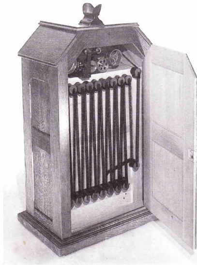
12.1 The Kinetoscope held film in a continuous loop threaded around a series of bobbins.
